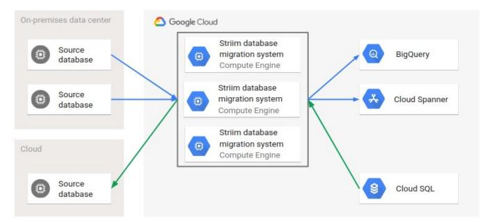
The direction of the data flow is reversed between the original source cloud database and Cloud SQL. After the migration is completed and the need for a fallback is ruled out, the related systems in
