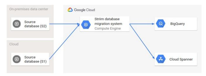
With the ability to transform and normalize data in streaming data pipelines, Striim can integrate a selected subset of the source transactional data to analytics platforms while the remaining data is continuously moved to one or more Google Cloud data targets.
